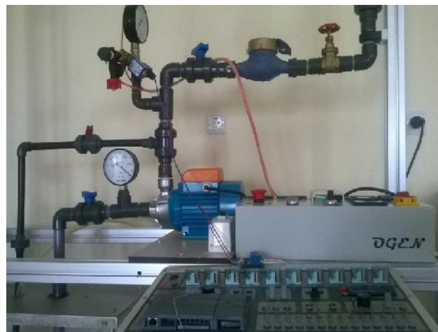
Figure 1. Centrifugal pump test bench
