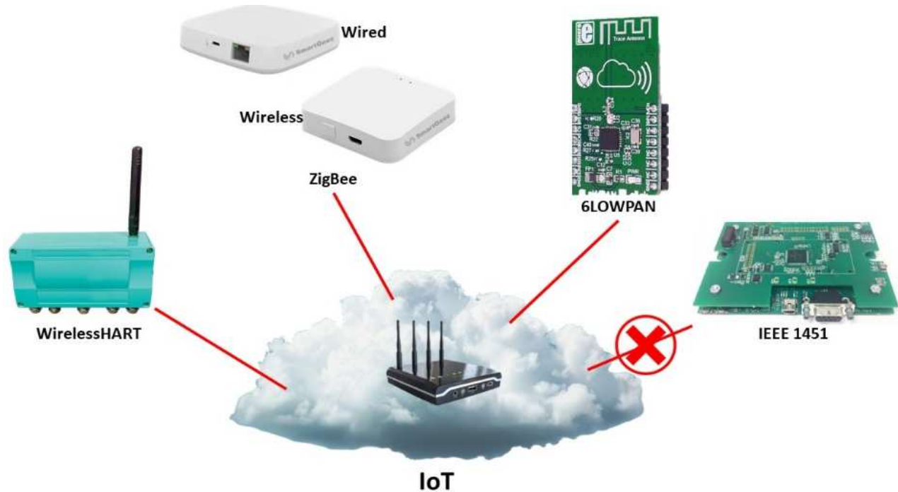
Figure 4. Smart network with smart gateway, comprised wireless highway addressable remote transducer, ZigBee, and 6LOWPAN.
