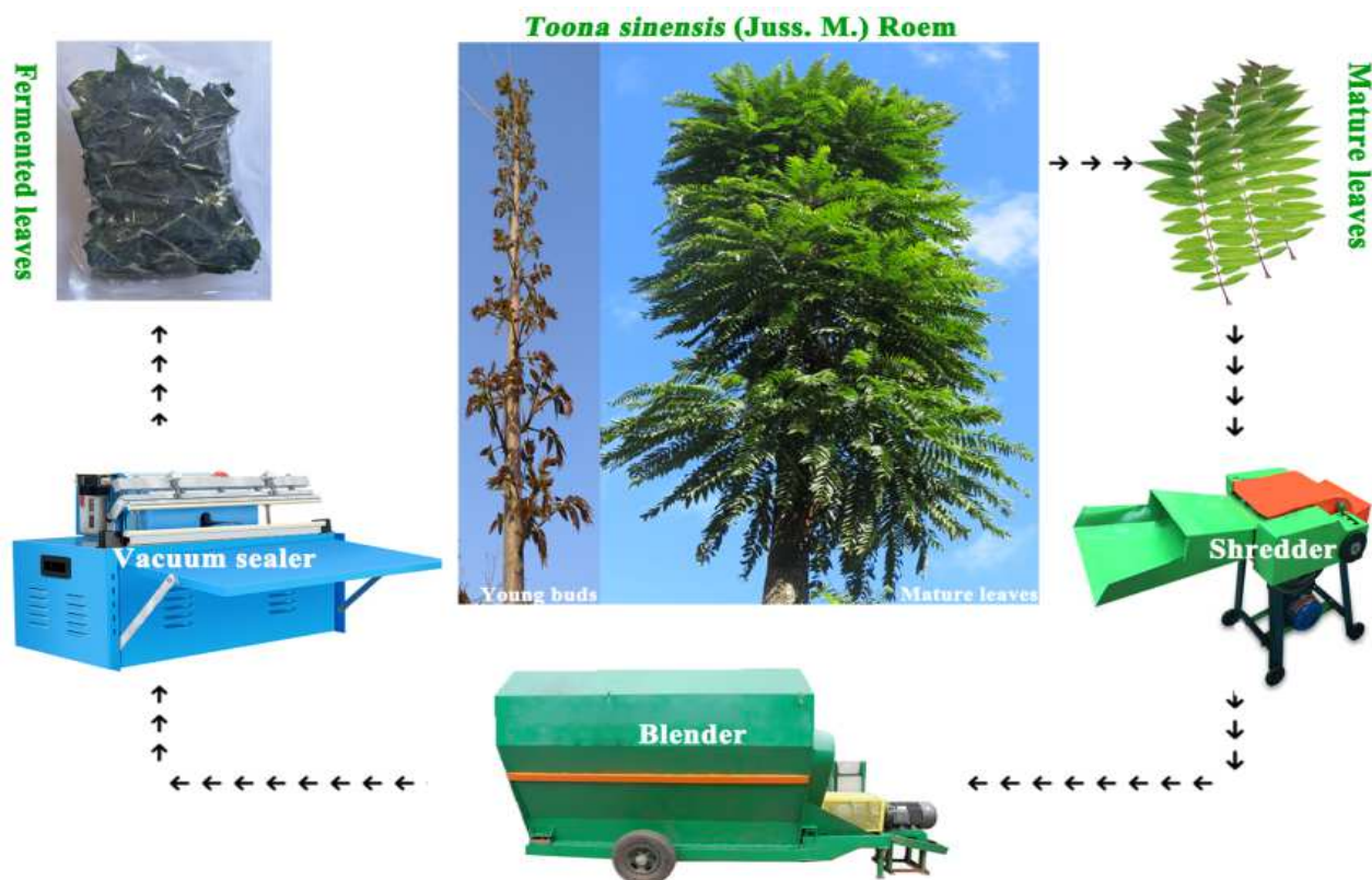
Fig. 1. Schematic diagram of the making process of fermented mature leaves of T. sinensis .
