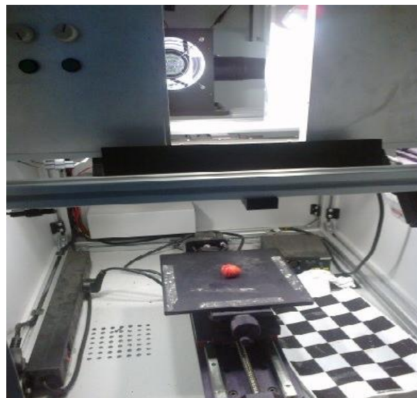
Figure 2. HyperSIS hyperspectral imaging system
