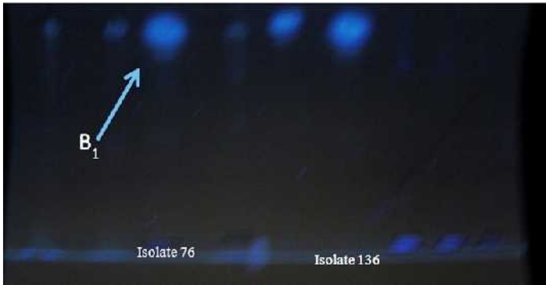
Figure 3: Thin layer chromatograph for Aspergillus flavus showing B 1
