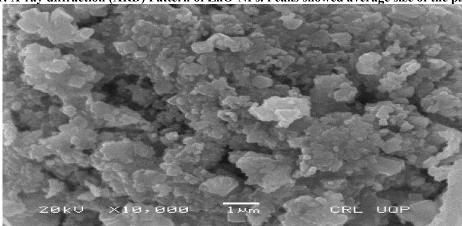
Fig. 2: Scanning electron microscopy (SEM) result of ZnO nanoparticles.
