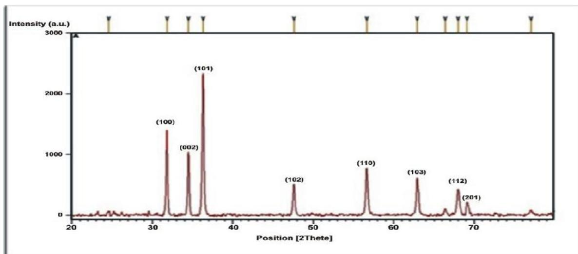
Fig. 1: X-ray diffraction (XRD) Pattern of ZnO-NPs. Peaks showed average size of the particles
