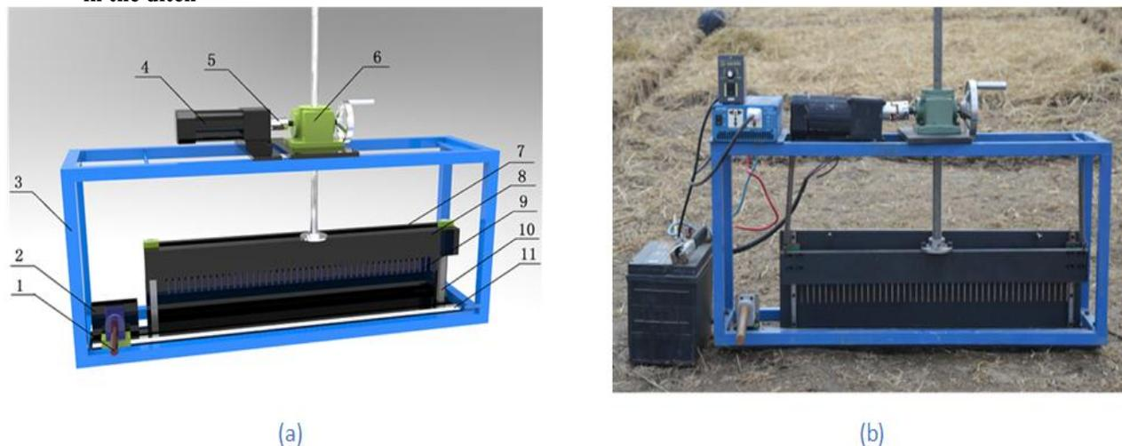
**Fig. 3. (a) Pro/E model of precision punch seeder (electrically powered), (b) The in-situ state of precision punch seeder 1. Handle 2. Seedbox 3. Frame 4. Drive motor 5. Coupling 6. Lifting mechanism 7, grid plate 8. Pressure plate 9. Pressure lever 10. Vertical rail 11. Horizontal rail**
