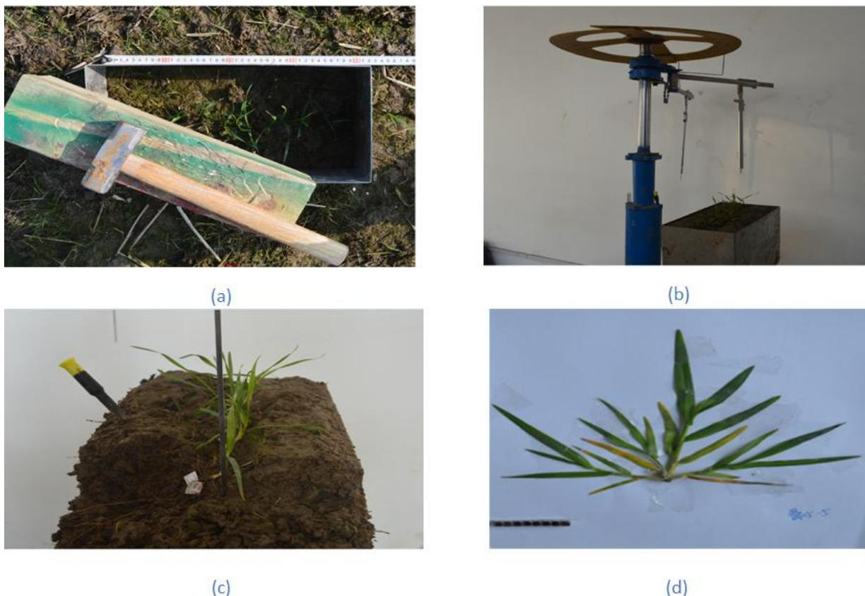
**Fig. 2. (a) Hammer and soil sampling cylinder, (b) Three-dimensional root configuration digitizer (c) Exploration of the root system of seedlings, (d) Acquisition of the leaf area**
