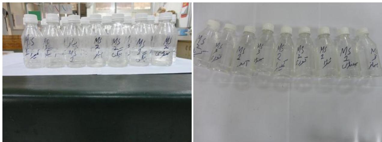
Figure 2. Vegetable samples after wet digestion for determination of heavy metal.
