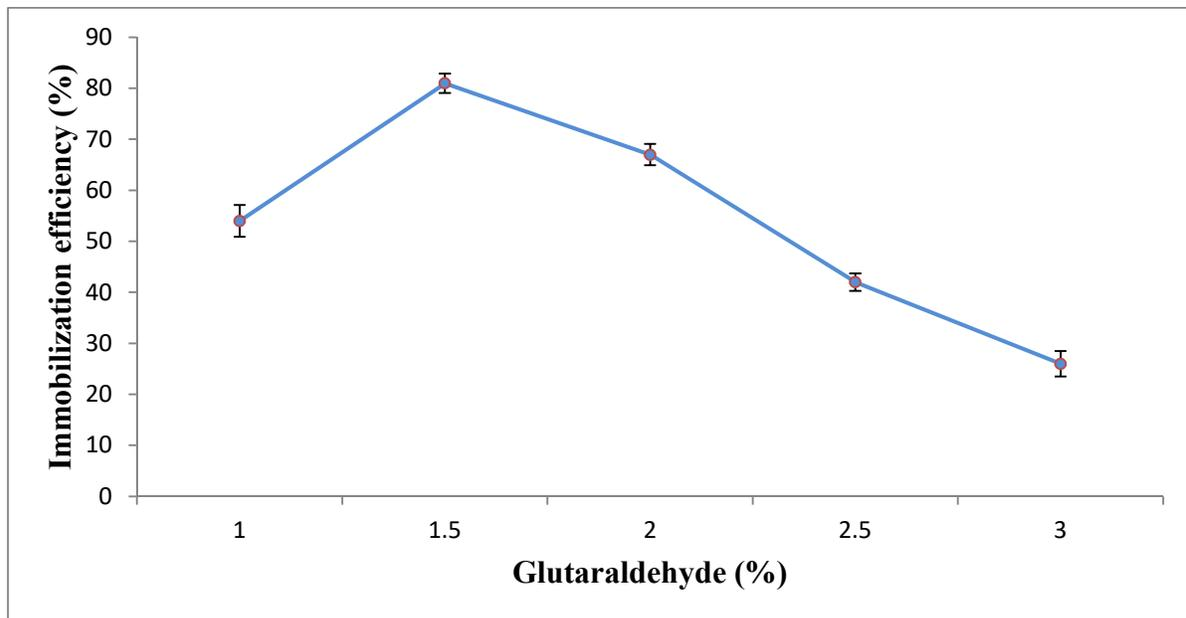
Fig. 2. Effect of different concentrations of Glutaraldehyde on laccase immobilization efficiency.
