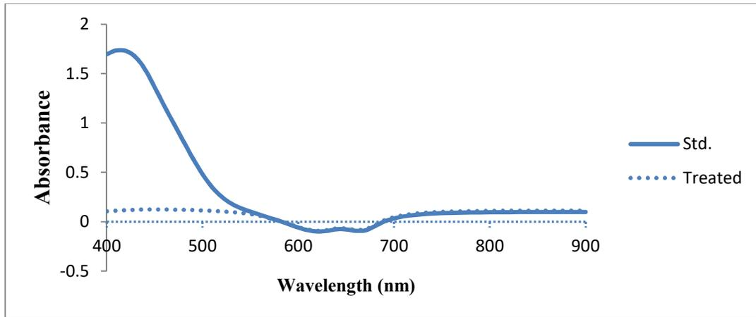
Fig. 10. UV-vis absorption spectra of S.F. GoldenYellow CRL dye after treatment with chitosan linked laccase from *P. ostreatus* IBL-02
