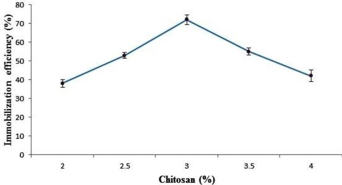
Fig. 1. Effect of different concentrations of Chitosan on laccase immobilization efficiency.
