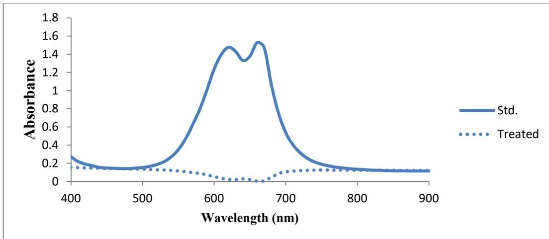
Fig. 12. UV-vis absorption spectra of S.F. Turq Blue GWWF dye after treatment with chitosan linked laccase from *P. ostreatus* IBL-02
