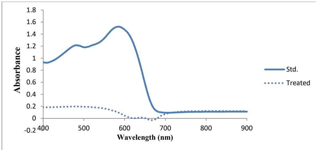
Fig. 11. UV-vis absorption spectra of S.F. Black CKF dye after treatment with chitosan linked laccase from *P. ostreatus* IBL-02
