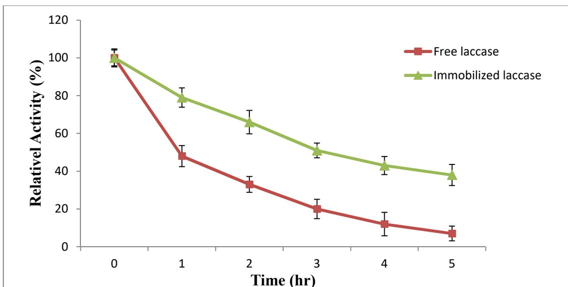
Fig. 7. Thermal stability of free and chitosan linked laccase at 60 °C.
