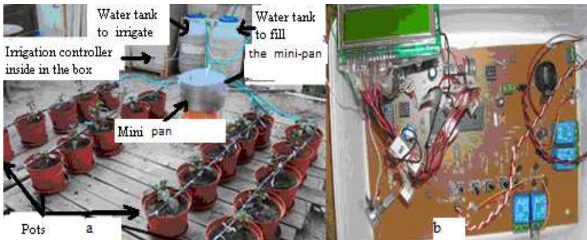
Figure 3. Layout of the experiment's components(a) and irrigation controller (b).
