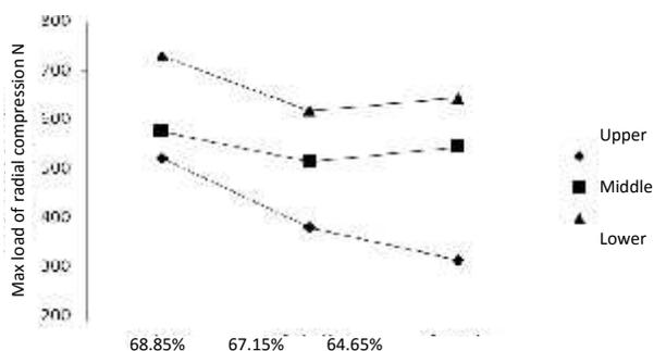
**Fig. 11** Effect of factors on maximum load of cassava stalks in radial compression
