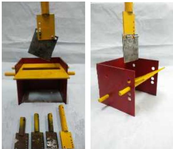
(a) Sliding cutting tools and support (b) Cutting tools and support
