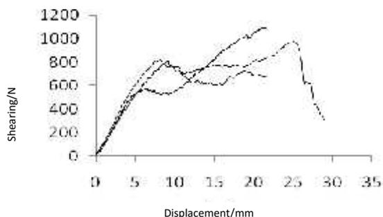
Fig. 14 The curve of load-displacement for sliding cutting test
