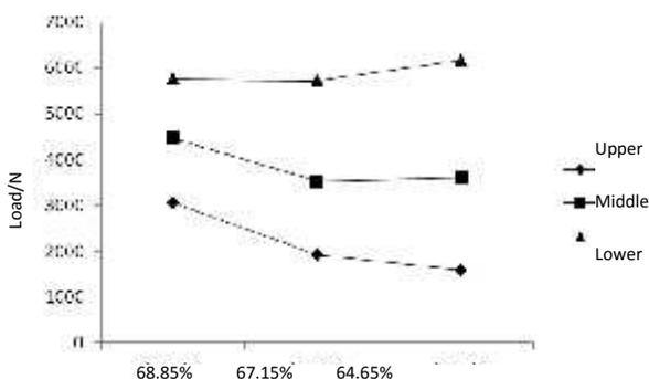
**Fig. 8. Effect of factors on maximum load of cassava stalks during axial compression**
