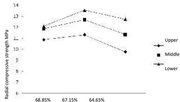
**Fig. 9. Effect of factors on axial compressive strength of cassava stalks**
