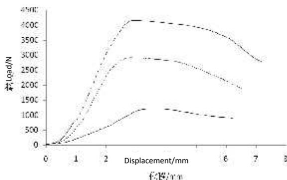
**Fig.7. The curve of load-displacement for the axial compression test**
