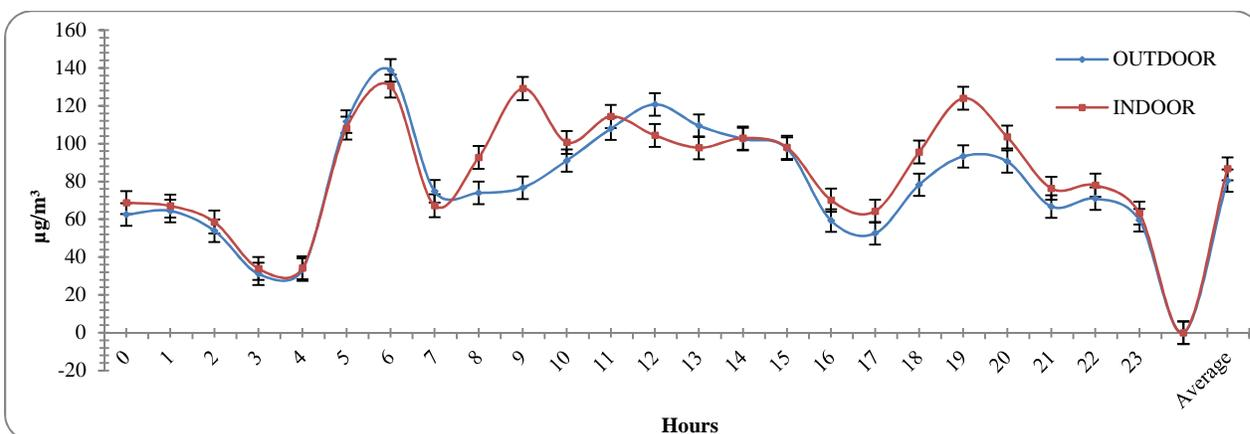
**Figure 1: Representative hourly average of indoor and outdoor PM<sub>2.5</sub> under high ventilation scenario**
