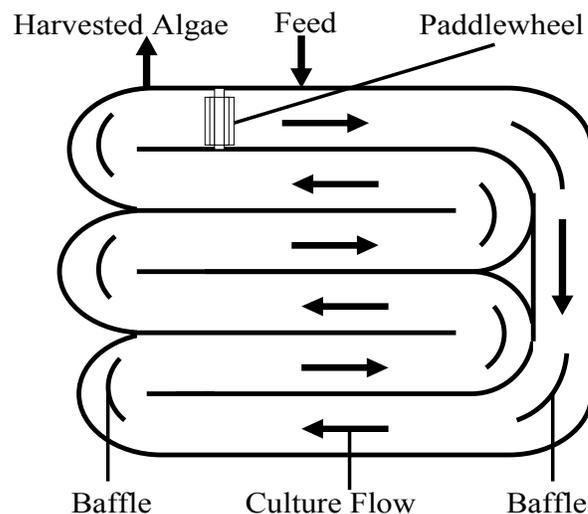
Figure 1. Schematic open pond system for *Cryptocodinium cohnii* culture.
