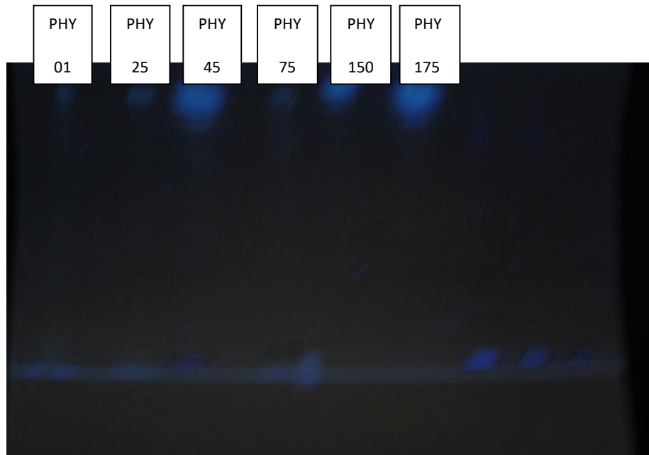
Fig. 2. Thin layer chromatogram of aflatoxins produced by toxigenic phytase producing isolates
